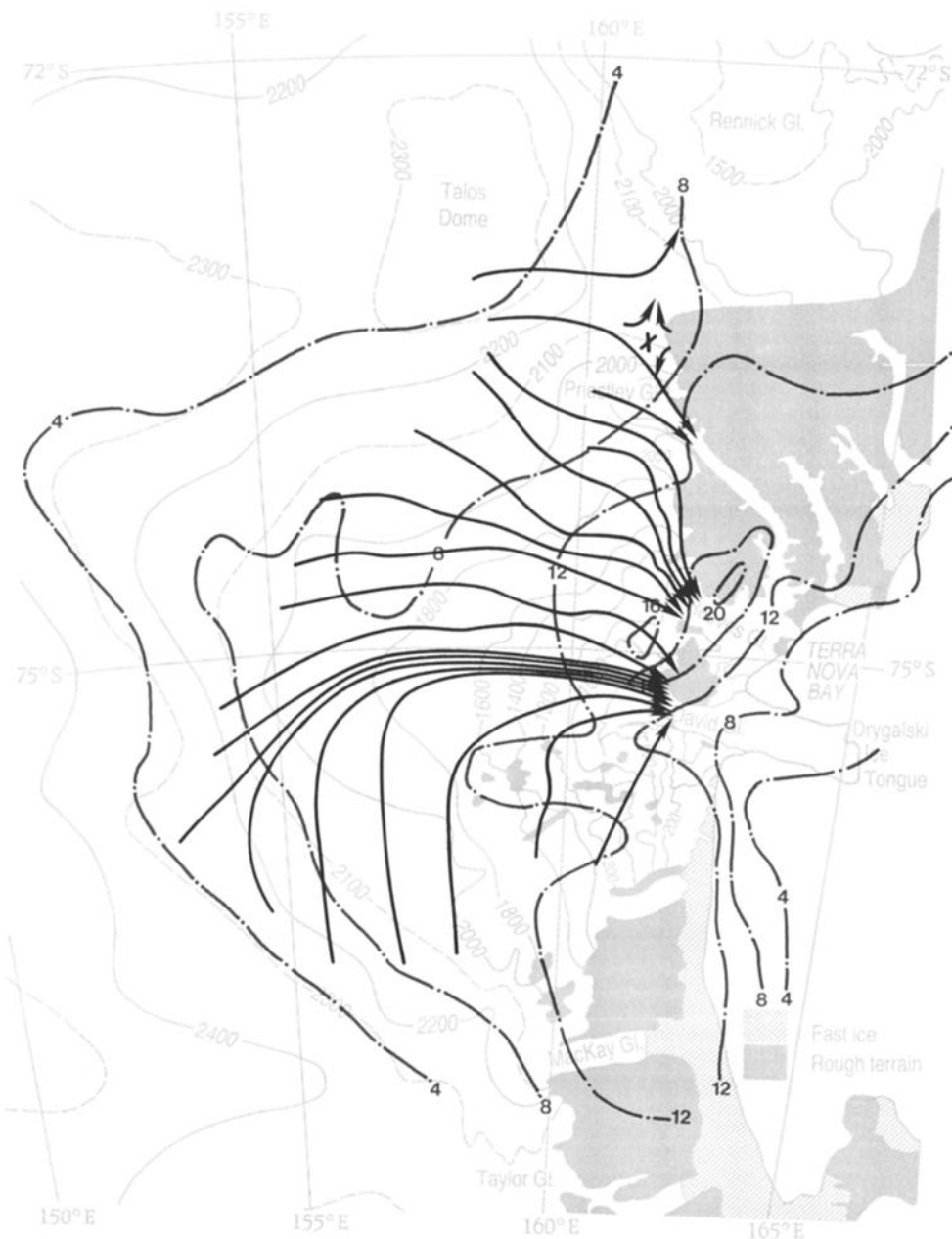
Fig. 9. Inferred streamlines (heavy continuous lines) compared with primitive equation surface-wind speeds in \text{m s}^{-1} (heavy dot-dash).
