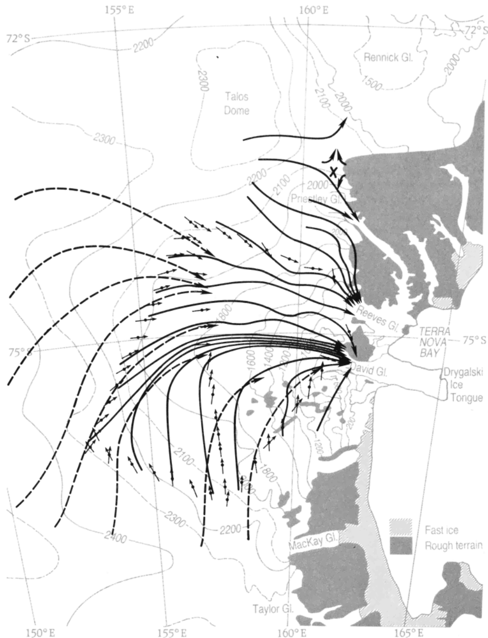
Fig. 7. Comparison between inferred streamlines of surface air motion (heavy solid lines) and those modeled by Parish and Bromwich [1987] (heavy dashed lines). Primary sastrugi directions are plotted at the centerpoint of every tenth 1987 photograph.
